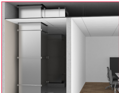
✗ The need for large air ducts for supply and exhaust, mechanical shaft space demand, results in large non-commercialized spaces
